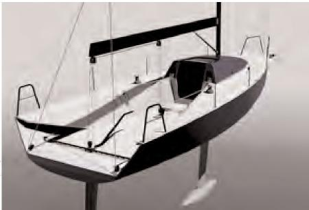
maximise the dynamic waterline and dynamic wavelength, resulting in a boost in upwind performance in displacement mode.
